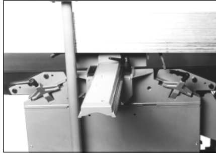
Loosen both clamping brackets and swing clear of the table brackets.
